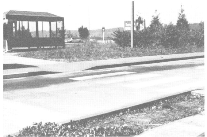
Fig. 5. Physical damage to the planting bed adjacent to the bus shelter directly corresponded to the observed traffic patterns shown in Figure 4. People using the parking lots tended to follow the provided sidewalks until a bus arrived at the stop. Then, they walked directly through any planting beds which intersected direct access to the bus.
